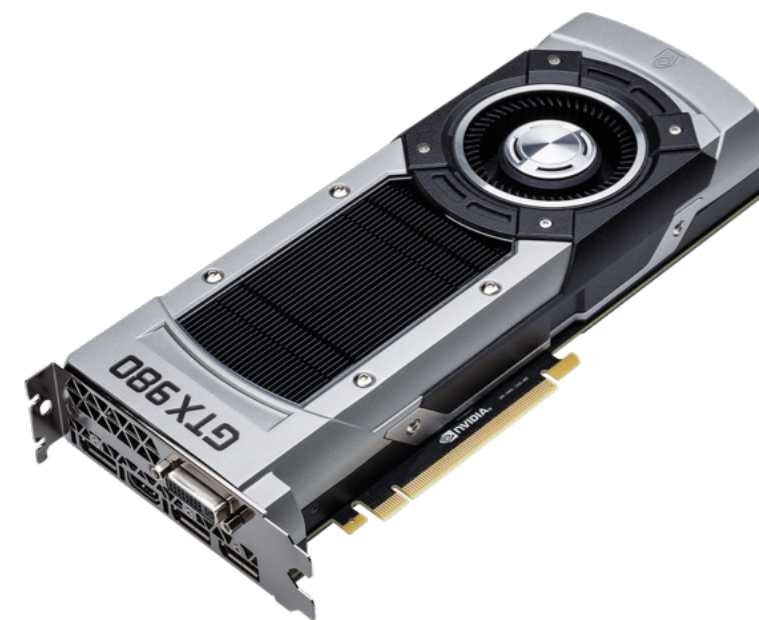
GTX 980: 16 SM cores (165 watts)
