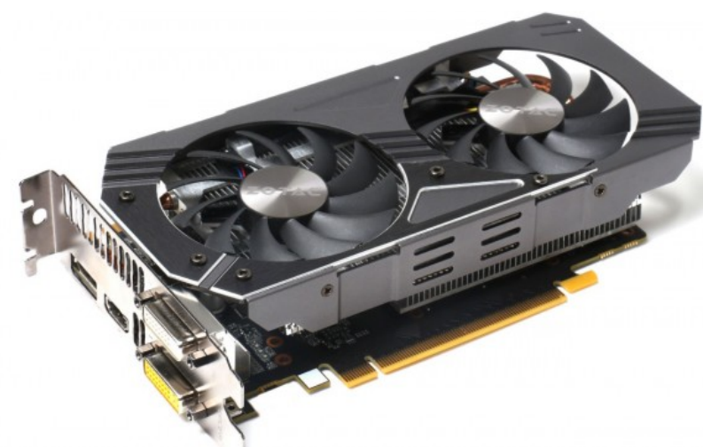
GTX 950: 6 SM cores (90 watts)
