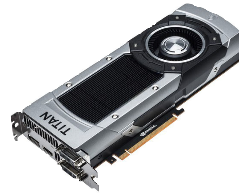
Titan X: 24 SM cores (250 watts)
