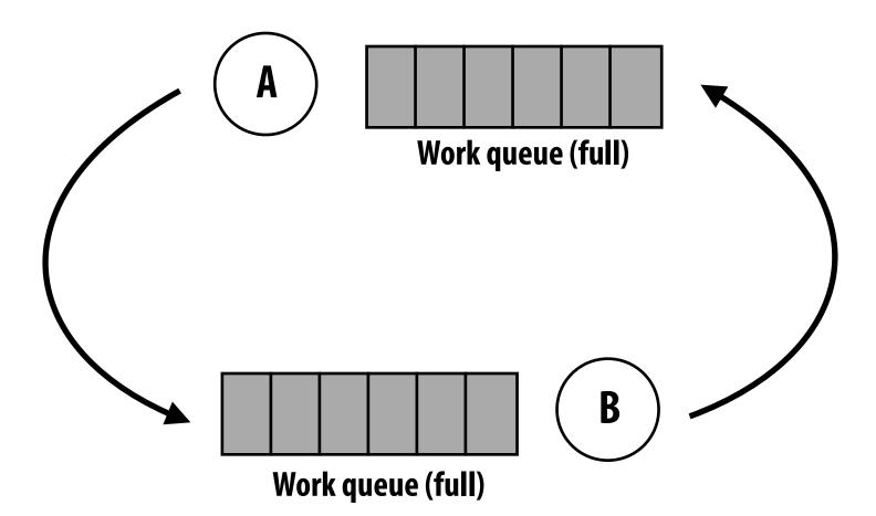
Thread A produces work for B's work queue
