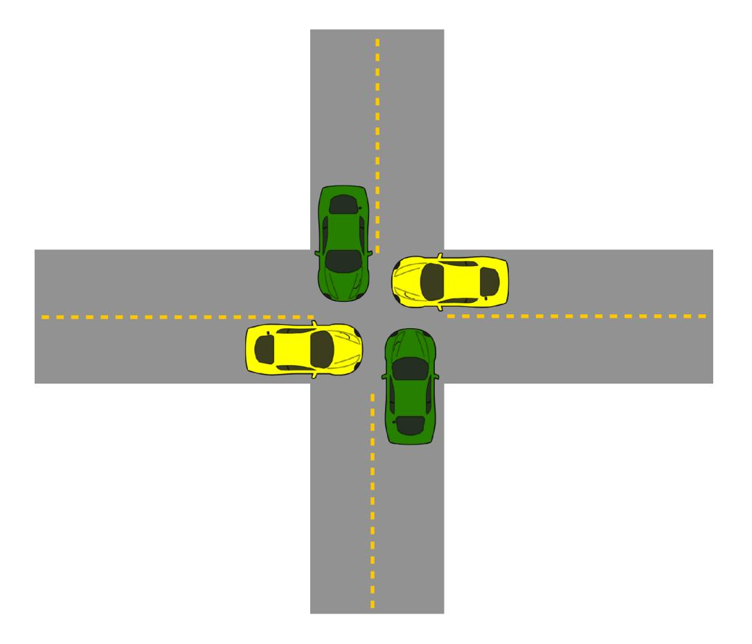
Deadlock is a state where a system has outstanding operations to complete, but no operation can make progress.
